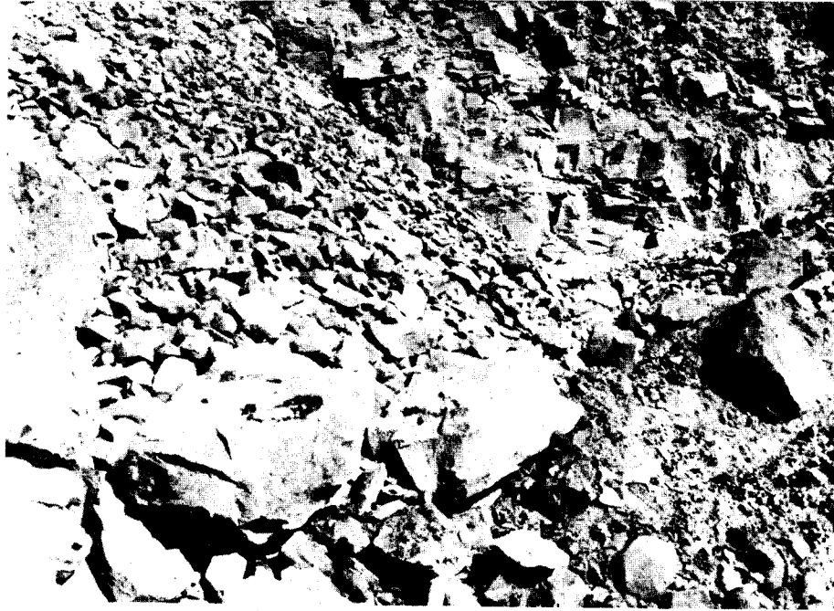
Plate 5.1. Blasted durable rock along highwall. Note the gradation of particle sizes available for both riprap and filter materials.
